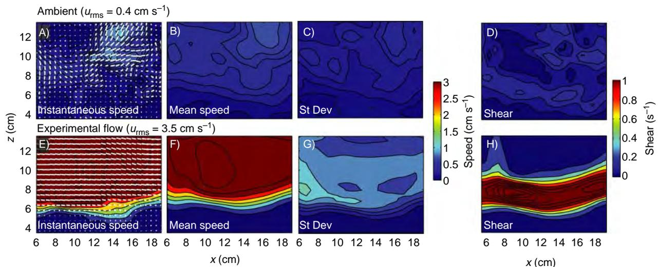
**Fig. 2** Ambient (A–D) and experimental flow (E–H) conditions from DPIV data. Velocity vectors and contours of speed magnitude from a representative pair of video frames are shown in A and E. Mean speed ( $s$ ) is shown in B and F, standard deviation in C and G, and shear rate ( $\gamma$ ) contours in D and H (see text for details). The field of view has been rotated so that the substratum is at the bottom of the frame.
