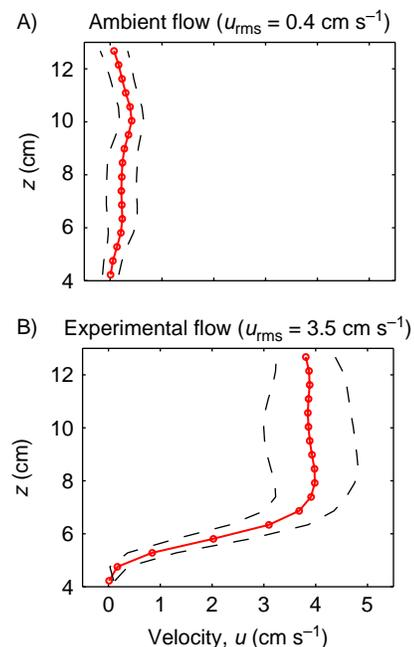
**Fig. 3** Mean water velocity profiles (red) relative to the surface of the substratum in ambient (A) and experimental (B) flow conditions. Vertical profiles were extracted from the DPIV data at the horizontal position  $x = 11.6$  cm. Velocity was measured over 14.3 s in ambient flow and 21.0 s in experimental flow. The dashed lines show the standard deviation of the mean velocity.
