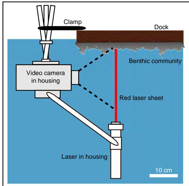
**Fig. 1** Side-view schematic of SCUVA setup under floating dock in Kaneohe Bay, Oahu, Hawaii. Dashed lines indicate the camera field of view; scale bar is shown at the lower right. The direction of flow in the experimental flow treatment is into the page. Note that the dock extends beyond the diagram to the right.
